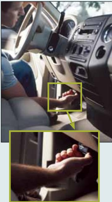
CarChip Pro plugs instantly and unobtrusively into the OBD II port in your car or truck.
