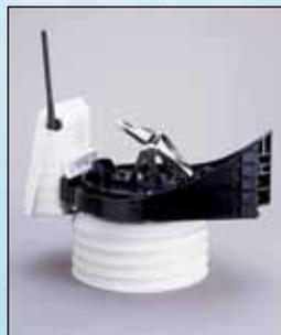
The aluminum-plated tipping bucket in our rain collector is self-emptying, corrosion resistant, and laser calibrated for exceptional accuracy.
