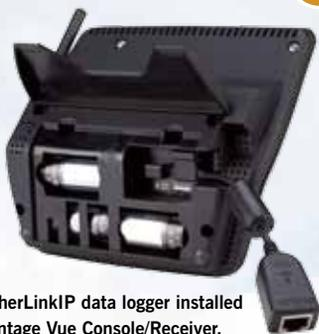
WeatherLinkIP data logger installed in Vantage Vue Console/Receiver.
