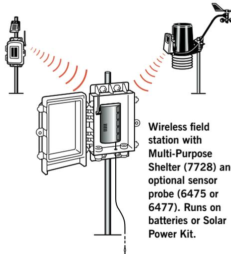
Wireless field station with Multi-Purpose Shelter (7728) and optional sensor probe (6475 or 6477). Runs on batteries or Solar Power Kit.
